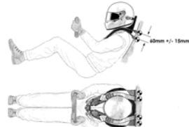
Figure 6. Installation of HANS® double belts in cars where (X < 200mm)
